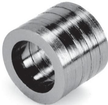
The K80STA is as a packing unit with two K80S antiextrusion rings (graphite with stainless steel sheet inserts) and three K80TA gaskets (flexible graphite with PTFE) from the MPA in Stuttgart with certificate no. 0010/2009 classified as high-quality packing within the meaning of the TA-Luft for temperature ranges greater than or equal to 250°C.
